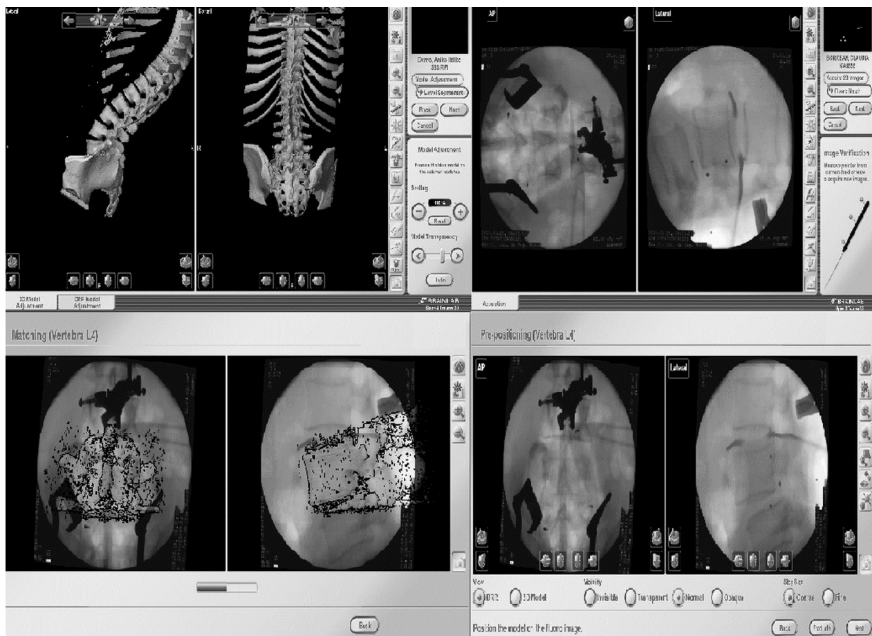
Figure 1: Fusion between the intraoperative fluoroscopy and a 3D model of a vertebra (based on the CT scan) and subsequently registration of the defined vertebra.
